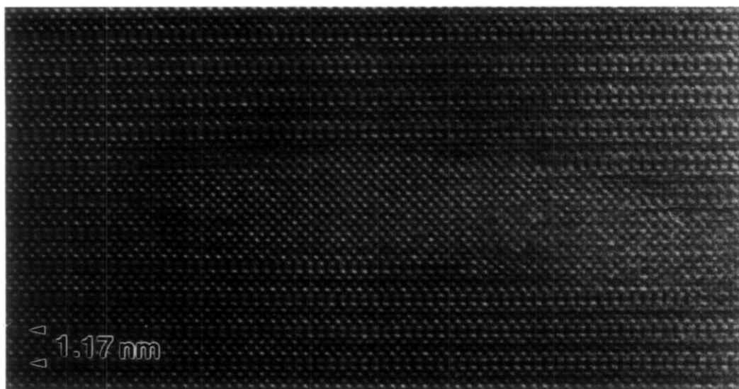
FIG. 5. A [110] micrograph recorded at a defocus value of about -80 nm showing an \text{Sr}(\text{Nb,Cu})\text{O}_3 intergrowth in \text{Sr}_2\text{NdNbCu}_2\text{O}_8 .
