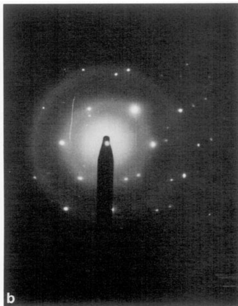
FIG. 3. TEM micrographs of as-prepared \text{LaCrO}_3 (a) agglomerate and (b) an electron diffraction pattern.
