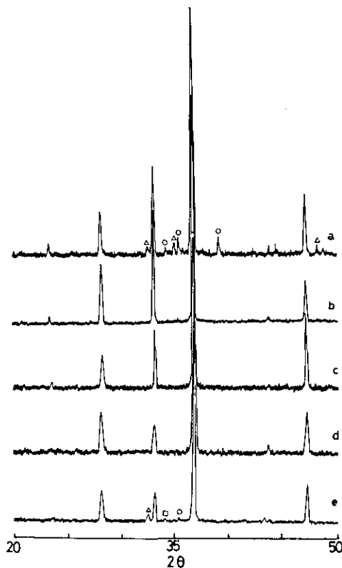
FIG. 1. X-ray diffraction patterns of powdered samples with the nominal composition \text{Ca}_{1-x}\text{Sr}_x\text{CuO}_2 fired at 1000^\circ\text{C} under flowing oxygen. x : 0.06 (a), 0.09 (b), 0.11 (c), 0.14 (d), and 0.16 (e). Peak assignment: \circ , \text{CaCu}_2\text{O}_3 ; \triangle , \text{Ca}_2\text{CuO}_3 ; \square , \text{Sr}_2\text{CuO}_3 ; none, layered solid solution.
