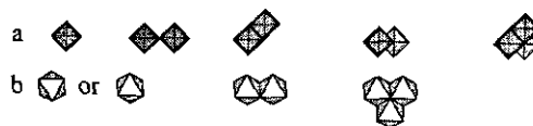
FIG. 1. Representation of Ti and (Ti, Me) octahedra for (a) Body centered cubic packing of anions. The darker octahedra are in the upper level of a two-level layer. (b) Hexagonal close packing of anions, showing corner and edge sharing of octahedra.
