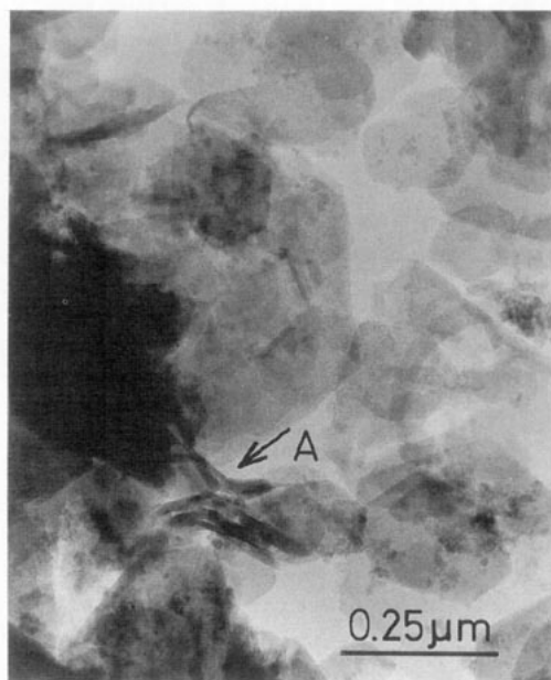
FIG. 4. TEM image from preparation 2, a sample which was nearly pure valleriite. Thin, platy valleriite crystals compose the bulk of this sample. The region arrowed "A" is enlarged in Fig. 6a.
