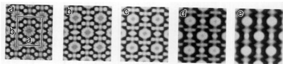
FIG. 1. Simulated images of MOR along [001] with different magnitude of the vibration parameter (VIB) used in the SHRL1 programs. The focus is 500 Å and the thickness is 45 Å. (a) VIB = 0 Å, (b) VIB = 0.4 Å, (c) VIB = 0.8 Å, (d) VIB = 1.2 Å, and (e) VIB = 1.6 Å. Images calculated with VIB = 0.8 Å correspond most closely to the experimental micrographs. The unit cell is outlined ( $a = 18.1$  Å and  $b = 20.5$  Å).
