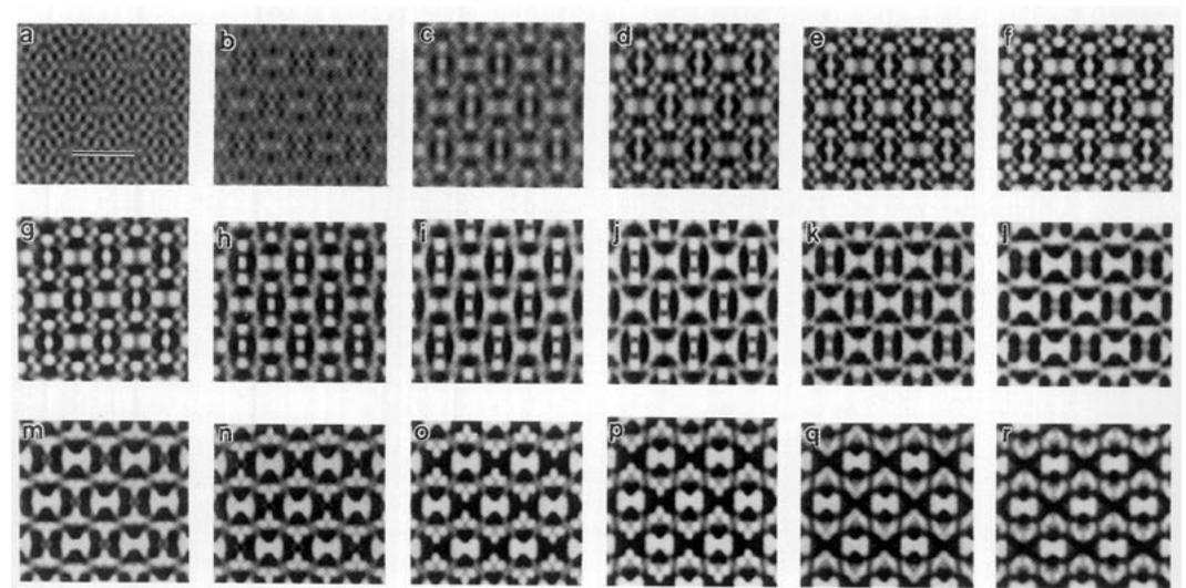
FIG. 10. Simulated images of FAU, with iron clusters in the center of the supercell, along [110], calculated for a thickness of 44 Å. The following focuses are calculated (a) 0, (b) 100, (c) 200, (d) 300, (e) 400, (f) 500, (g) 600, (h) 700, (i) 800, (j) 900, (k) 1000, (l) 1100, (m) 1200, (n) 1300, (o) 1400, (p) 1500, (q) 1600, and (r) 1700 Å. The images are very different from the ones without iron clusters (Fig. 7), except at focuses close to 1100 Å. Scale bar = 15.2 Å.
