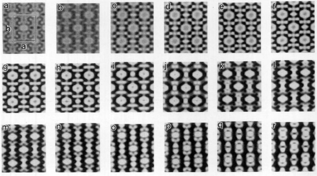
FIG. 4. Simulated images of MOR along [001] at a crystal thickness of 45 Å and the following focuses (a) 0, (b) 100, (c) 200, (d) 300, (e) 400, (f) 500, (g) 600, (h) 700, (i) 800, (j) 900, (k) 1000, (l) 1100 (m) 1200, (n) 1300, (o) 1400, (p) 1500, (q) 1600, and (r) 1700 Å. The dark spots which are obvious at focuses close to 500 Å are gone at 1000 Å. Still lower focuses give images where the channels are easily discerned. The unit cell is outlined ( $a = 18.1$  Å and  $b = 20.5$  Å).
