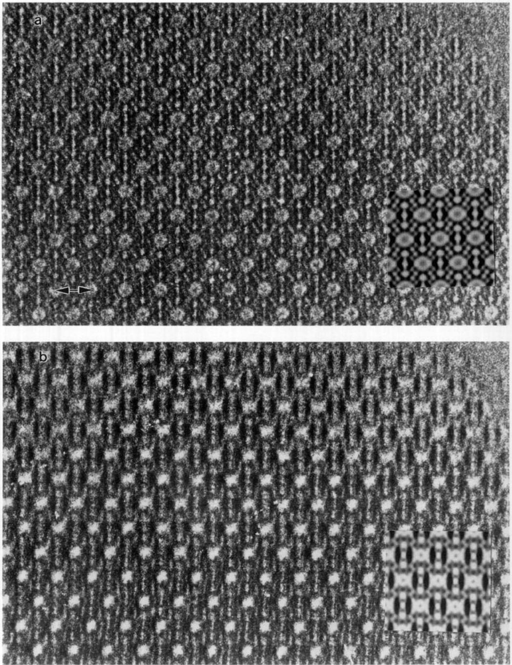
FIG. 6. Micrographs of a FAU crystal recorded at two focus values, approximately 500 (a) and 1000 Å. (b). Inserted are the simulated images at these focuses calculated for a thickness of 44 Å. The micrograph at 1000 Å, taken after the one at 500 Å, is damaged by the electron beam. The beam incidence is [110]. Scale bar = 15.2 Å.
