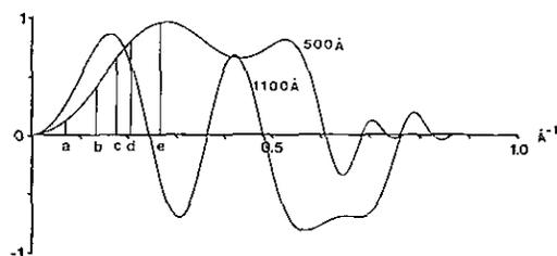
FIG. 8. The CTF for 500 and 1100 Å. The location of the Bragg reflections for FAU listed in Table III (a, b, c, d and e) are marked. At 1100 Å the c- and d-reflections (D) have a poorer transfer than at 500 Å while the others are more strongly transferred.
