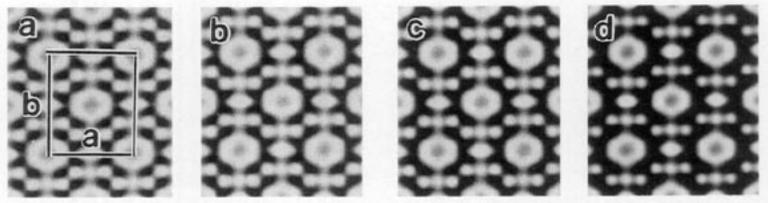
FIG. 2. Simulated images of MOR along [001] at a defocus of 500 Å for different thicknesses. (a) 15, (b) 45, (c) 75, and (d) 105 Å. The images do not change significantly in this rather large thickness interval. Further simulations were made for both zeolites at a thickness of about 45 Å. The unit cell is outlined ( $a = 18.1$  Å and  $b = 20.5$  Å).
