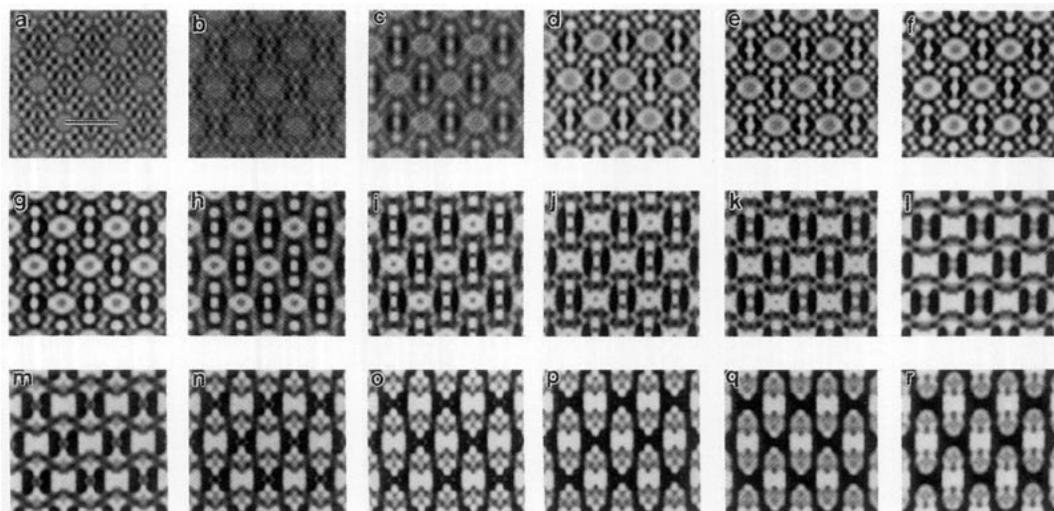
FIG. 7. Simulated images of FAU along [110] calculated for a crystal thickness of 44 Å and the focuses (a) 0, (b) 100, (c) 200, (d) 300, (e) 400, (f) 500, (g) 600, (h) 700, (i) 800, (j) 900, (k) 1000, (l) 1100, (m) 1200, (n) 1300, (o) 1400, (p) 1500, (q) 1600, (r) 1700 Å. The spots in the channels remain visible down to a focus of 1000 Å after which the appearance of the images changes drastically. Scale bar = 15.2 Å.
