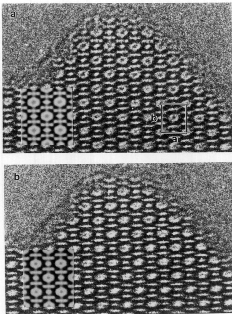
FIG. 3. Micrographs of a crystal of MOR recorded with the electron beam parallel to [001]. The focus values are approximately 500 (a), 700 (b), and 900 Å (c). Inserted are the simulated images at these focuses calculated for a thickness of 45 Å. The crystal gets thicker very quickly so only the edge is interpretable. The spot contrast weakens when the focus is lowered. The unit cell is outlined ( $a = 18.1 \text{ \AA}$  and  $b = 20.5 \text{ \AA}$ ).
