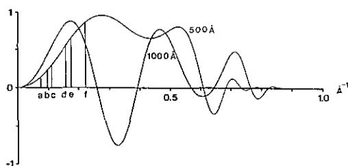
FIG. 5. The CTF calculated for 500 and 1000 Å. The location of the Bragg reflections for MOR listed in Table II (*a*, *b*, *c*, *d*, *e*, and *f*) are marked. All reflections except *f* are more strongly transferred at 1000 than at 500 Å. The *f*-reflection, which is the most important D-reflection, is, however, weaker. This results in the fact that the dark spot is absent at this focus.
