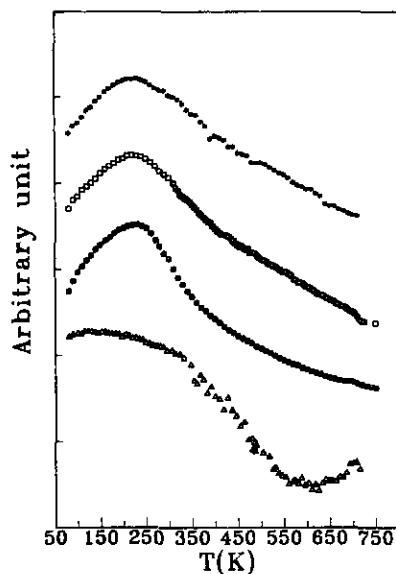
FIG. 11. Normalized resistivity vs temperature for Y_xBa_{2-x}Nb_5O_9 ( x = 0.00, 0.05, 0.10, 0.20 from bottom to top). Resistivity is plotted on a linear scale
