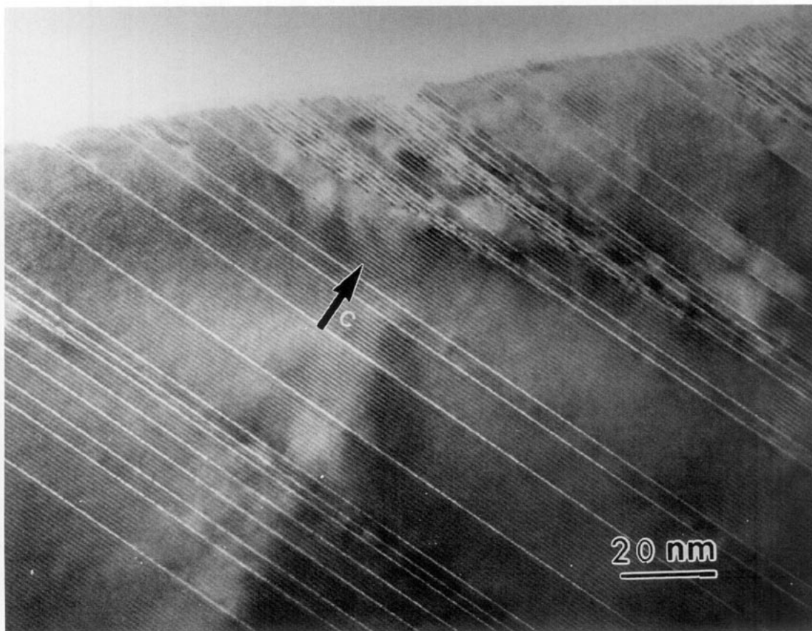
FIG. 3. Transmission electron micrograph of the \text{Li}_{.26}\text{Ba}_2\text{PrCu}_3\text{O}_7 sample taken along the [010] zone axis. Extended defects perpendicular to the c^* axis of the 123 matrix are clearly observed.
