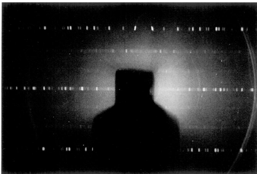
PHOTOGRAPH 1. The Bragg X-ray photograph of \text{Gd}_{2/3}\text{Cr}_2\text{S}_4 showing the a lattice spacing. The strong reflection lines correspond to the lattice spacing of a = 3.50 \text{ \AA} . The weaker reflections correspond to the 3a superstructure.
