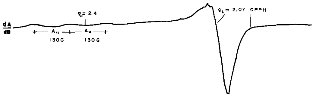
FIG. 3. X-band (9.204 GHz) EPR spectrum of DMSO frozen solution of [\text{Cu}(\text{HL})(\text{OH}^-)]_n at 77 K.
