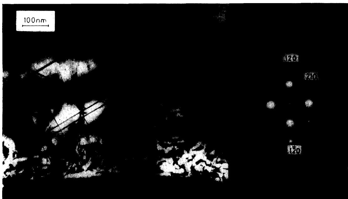
FIG. 2. An 001 section showing isolated boundaries of all four possible {210} orientations in TiO 2 2% FeO 1.5 .
