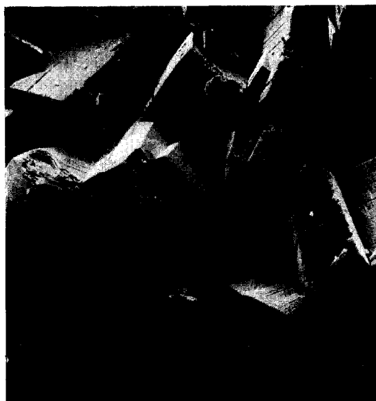
Fig. 5. Scanning electron micrograph of molybdenum trioxide, pseudomorphous after molybdenum trioxide-dihydrate. Orientation of lamellae: (010). 130 \times .
