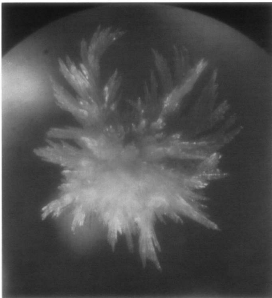
FIG. 10. Coarse spherulite of \beta - \text{Cu}(\text{IO}_3)_2 growing on small sphere of \alpha - \text{Cu}(\text{IO}_3)_2 (overall diameter 4 mm).
