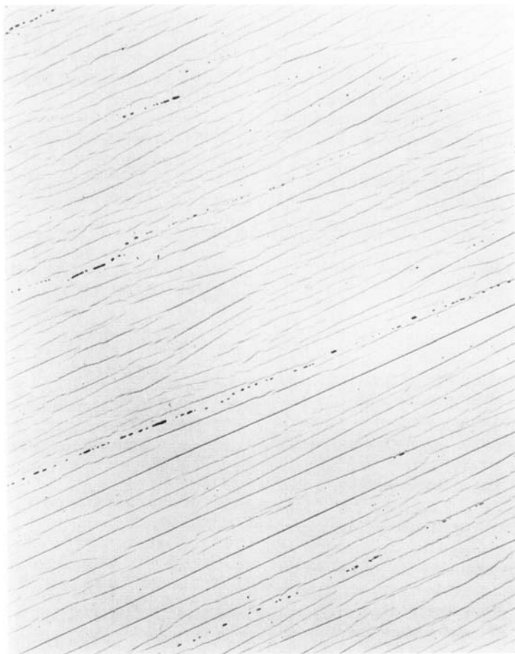
FIG. 7. Melt-grown Mn_nSi_{2n-m} annealed 50 hr at 1130°C, and quenched. The MnSi precipitate spacing is around 20 \mu m . Figure 3 depicts the as-grown material before the quench-anneal procedure. As polished, polarized light, \times 100 .
