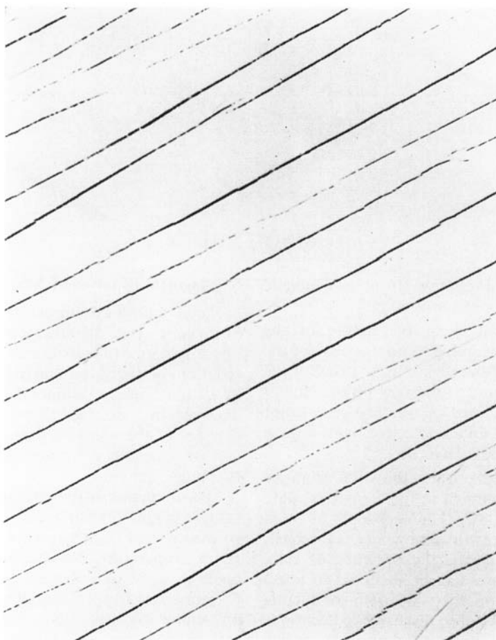
FIG. 3. As-grown \text{Mn}_n\text{Si}_{2n-m} "single crystal" containing plate-like precipitates of MnSi (dark lines) lying in the (001) plane of \text{Mn}_n\text{Si}_{2n-m} . The precipitate spacing is about 100\ \mu\text{m} . As polished sample, polarized light, \times 100 .
