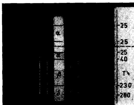
FIG. 5. \delta -Sr(HCOO) 2 temperature regulating X-ray diffraction pattern—25°C hr -1 cooling rate. (Lower pattern) \delta \rightarrow \beta \rightarrow \alpha transitions during the cooling of the sample in an open glass capillary. (Upper pattern) \alpha -Sr(HCOO) 2 diffraction lines at 25°C, the film moving for 4 hr without any heating.
