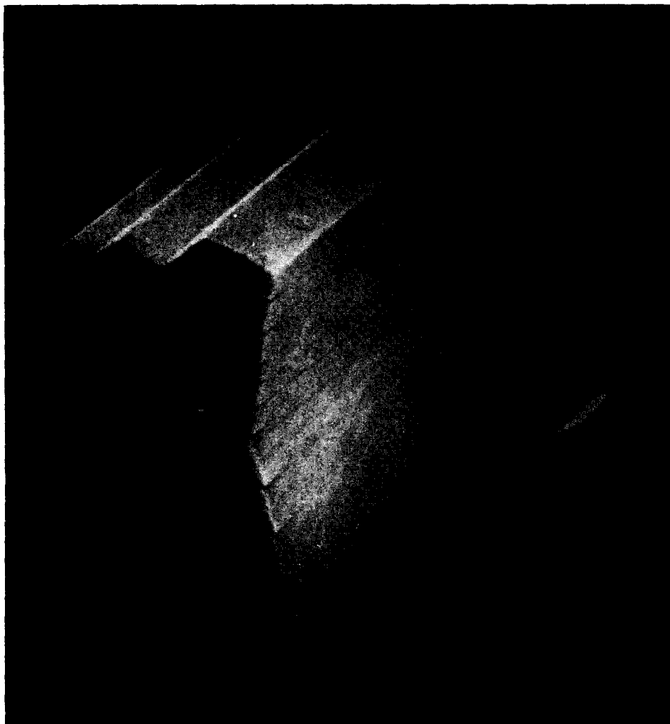
FIG. 4. Scanning electron micrograph of molybdenum trioxide, pseudomorphous after white molybdenum trioxide-monohydrate. Cracks are running parallel to [010]_{\text{MoO}_3 \cdot \text{H}_2\text{O}} ( \times 1440 ).
