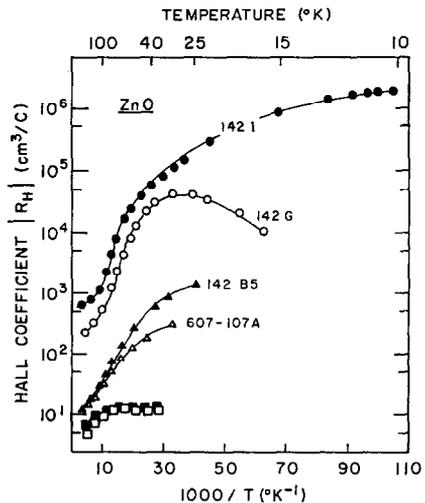
FIG. 2. Temperature dependence of Hall coefficient  $R_H$  from 10 to 300 K. An  $R_H$  maximum is clearly observed in sample 142G. □ 142A; ■ 145N.
