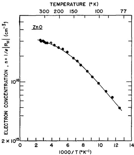
FIG. 4. Nonlinear least-square fit for sample 142G using values for  $E_D$ ,  $N_D$ , and  $N_A$  given in Table II. ( $\beta = 2$  or 0.5 give practically the same curve.) ● experimental; — nonlinear least-square fit.
