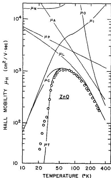
FIG. 5. Best fit to the Hall mobility data of sample 142G by using a two band model.  $\mu_c$  is the conduction band mobility calculated from lattice and defect mode scatterings; and  $\mu_T$  is the total mobility of the two band conduction model where  $\mu_{HDB} = 2 \text{ cm}^2 \text{ V}^{-1} \text{ sec}^{-1}$ .  $\circ$  = experimental.
