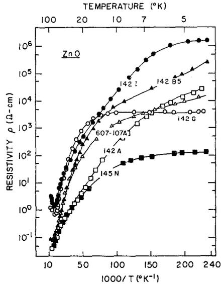
FIG. 1. The resistivity  $\rho$  is shown vs  $10^3/T(K^{-1})$  from 4.2 to 300 K.
