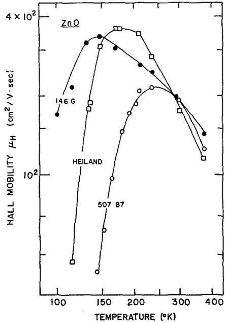
FIG. 3b. Temperature dependence of Hall mobility  $\mu_H$  for three highly resistive samples.
