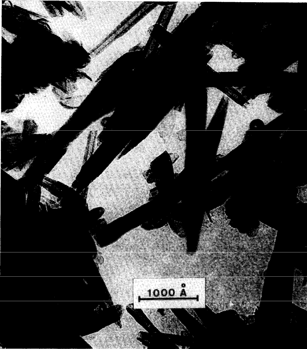
FIG. 3. Nickel antigorite with rolled sheets. \times 250,000 .
