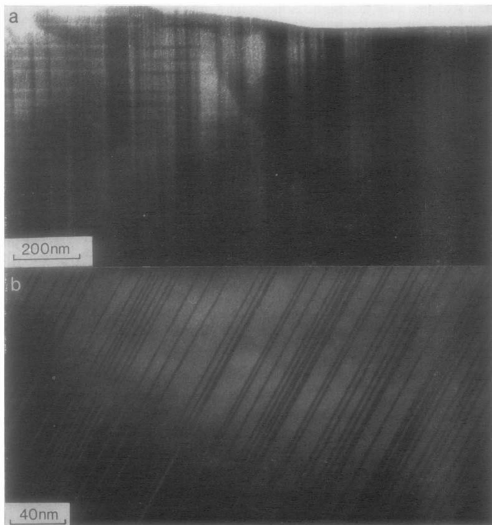
FIG. 4. (a) Micrograph taken from an arc-melted sample showing faults exhibiting poor interfacial contrast. (b) Micrograph taken from an annealed sample. The faults are sharper and more clearly delineated.
