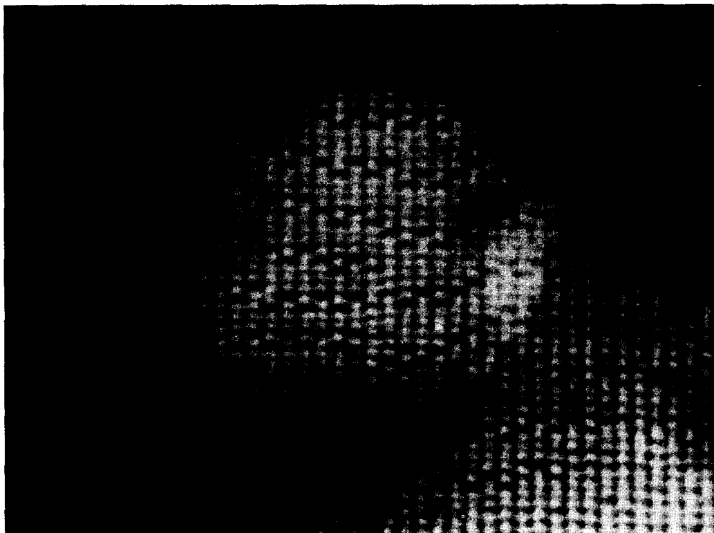
FIG. 9. Dislocation associated with termination of a (stepped) CS plane within the crystal.
