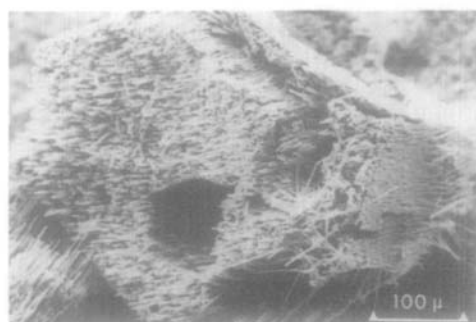
FIG. 3. Typical appearance of an HTB crystal which has been oxidized in air or oxygen.
