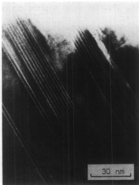
FIG. 2. Electron micrograph showing isolated groups of (121) CS planes in a \text{VO}_2 matrix.
