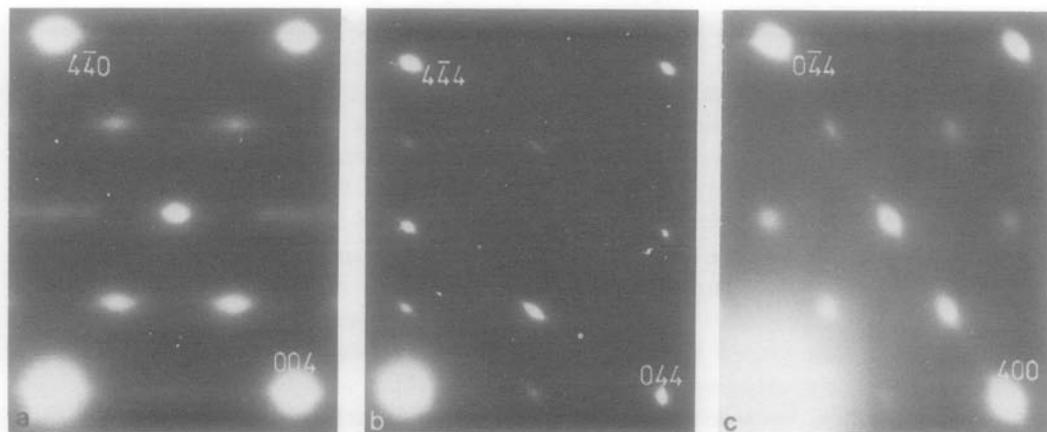
FIG. 4. Streaking effects in electron diffraction patterns from furnace-fired boehmite fragments exhibiting the lamellar porous microstructure. (a)  $[110]$ , (b)  $[21\bar{1}]$ , and (c)  $[011]$   $\gamma$ - $\text{Al}_2\text{O}_3$  zones.
