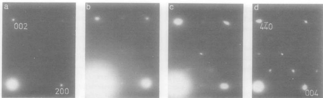
FIG. 2. Typical electron diffraction pattern sequence for electron beam-induced dehydration of boehmite, from (a)  $[010]_{\text{Bo}}$  to (d)  $[110]_{\gamma}$ .
