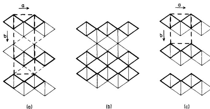
FIG. 1. Idealized structures of (a) boehmite, (b) collapsed boehmite (*ccp* lattice), and (c) FeOCl.
