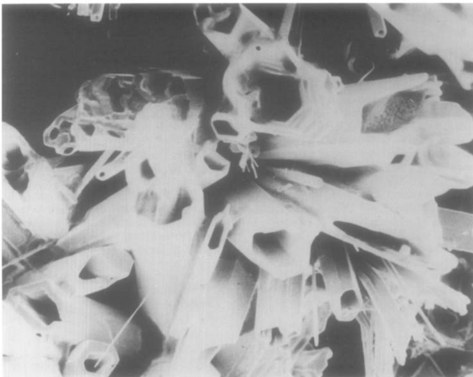
FIG. 8. VS_4 crystals grown by reaction of V_5S_8 with sulfur ( \times 100 magnification).
