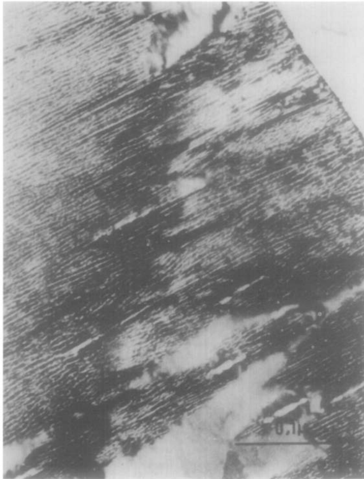
FIG. 1. Underfocused bright field image of a partly transformed goethite crystal in the G[010] orientation. Note the white striae consisting of rows of cavities which form a grating with a spacing of about 50 Å.
