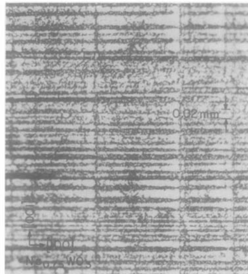
FIG. 11. Unpolarized-light photomicrograph of slightly etched (010) surface of \text{Na}_{0.75}\text{WO}_3 , showing the sodium segregation in a venetian-blind pattern. The sodium content is higher in the lighter area. The striations are parallel to the \langle 100 \rangle axes. This surface showed no optical birefringence. The surface was mechanically polished and then etched using the modified Murakami reagent at room temperature.
