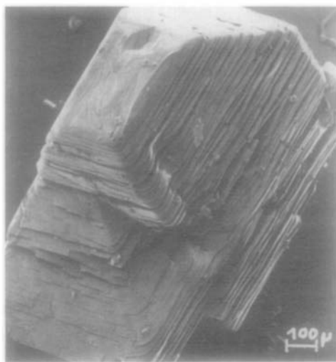
FIG. 1. Scanning electron micrograph of a dehydrated copper(II) formate tetrahydrate crystal, showing pronounced splitting parallel to the basal plane.
