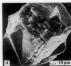
PLATE 1. Scanning electron micrographs of pristine \alpha -AlH 3 powder. (a) Overall view of the \alpha -AlH 3 cuboids: side lengths \sim 50–100 \mu m. Notice the variety of surface detail as well as the presence of several contact and interpenetration twinned crystals. (b) Close-up of a typical cuboid showing the presence of several surface pits. The remainder of the surface has a smooth, even appearance. The pits contain steps and layers. (c) Close-up detail of a typical surface pit showing the interior layer-like structure. Also, small sphere-like particles (0.05–0.4 \mu m in diameter) are shown adhering to all surfaces. (d) A simple, interpenetrating twinned cuboid crystal. Most twinned cuboids were considerably more complex than this example. (e) A drawing of an idealized penetration on twin with twin axis [001]. The twinned crystal (shaded) has been oriented to compare with (d). Also shown are the edge directions and habit faces of the cuboids determined from single-crystal X-ray analysis.
