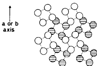
FIG. 1. Plan of the interlayer sites between the (\text{UO}_2\text{PO}_4)_n^- layers (after Ross and Evans (14)). The unshaded sites are elevated with respect to the shaded ones. The sites can be occupied by either water molecules or monovalent cations.
