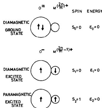
FIG. 2. Possible electronic excitations in oxide of high valence cation  $M^{(2n/m)+}$  with rare-gas-type outer electronic shell.
