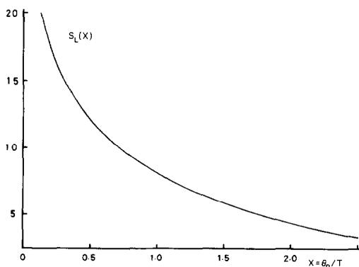
FIG. 1. Entropy  $S_L(x)$  in (cal/deg · g-atom) associated with lattice vibration is drawn as a function of  $x = \Theta_D/T$ .
