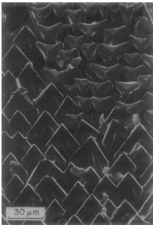
FIG. 5. Epitaxial grown NiTiO_3 crystals on the NiTiO_3 diffusion zone (SEM photograph).
