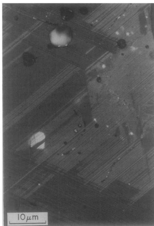
FIG. 3. Decomposed spinel sample due to retempering of a spinel at 1250°C. Oriented NiTiO 3 exsolution lamellae are intergrown with NiO. The NiO host crystal is cut nearly parallel {111} (reflected light photograph using polarized light and oil immersion).
