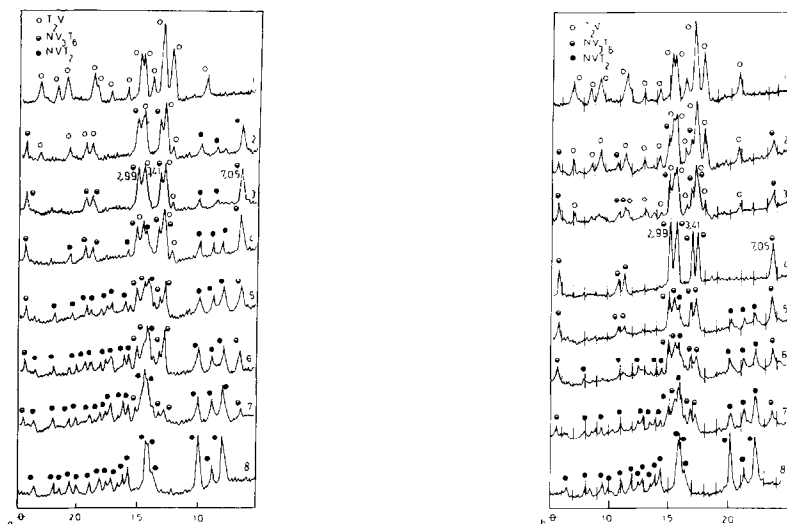
FIG. 1. X-Ray diffraction data on compositions in the T_2V\text{--}NVT_2 system. (a) Products prepared by solid-state reaction: (1) T_2V ; (2) 90T_2V \cdot 10NVT_2 ; (3) 70T_2V \cdot 30NVT_2 ; (4) 66.6T_2V \cdot 33.3NVT_2 ; (5) 50T_2V \cdot 50NVT_2 ; (6) 40T_2V \cdot 60NVT_2 ; (7) 20T_2V \cdot 80NVT_2 ; (8) NVT_2 . (b) Products prepared by crystallization of glasses: (1) 33.3V_2O_5 \cdot 66.6TeO_2 ; (2) 2.5 Na_2O \cdot 32.5V_2O_5 \cdot 65TeO_2 ; (3) 7.5Na_2O \cdot 30.8V_2O_5 \cdot 61.7TeO_2 ; (4) 10Na_2O \cdot 30V_2O_5 \cdot 60TeO_2 ; (5) 12.5Na_2O \cdot 29.2V_2O_5 \cdot 58.3TeO_2 ; (6) 15Na_2O \cdot 28.3V_2O_5 \cdot 56.7TeO_2 ; (7) 20Na_2O \cdot 26.7V_2O_5 \cdot 53.3TeO_2 ; (8) 25Na_2O \cdot 25V_2O_5 \cdot 50TeO_2 .
