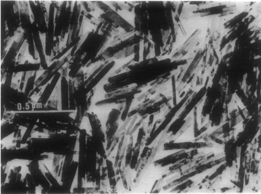
FIG. 2. Electron micrograph of the sample of CrO 2 with \tau = 0.362 \mu\text{m} . The acicularity ratio is of the order of 10/1 and the c axis is parallel to the longest dimension.
