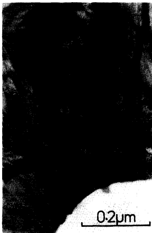
FIG. 2. Low-magnification electron micrograph of a typical crystal plate of the rhombohedral phase. The dark bands are extinction contours and indicate that the plate is bowed into either a saucer or a dome shape.
