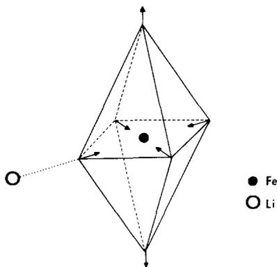
FIG. 2. Elongation of the  $\text{FeO}_6$  octahedron in  $\text{Sr}_{0.5}\text{La}_{1.5}\text{Fe}_{0.5}\text{Li}_{0.5}\text{O}_4$ .
