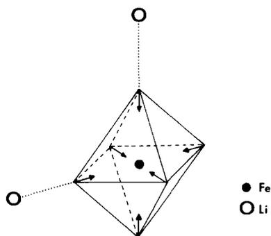
FIG. 3. Contraction of the  $\text{FeO}_6$  octahedron in  $\text{La}_2\text{LiFeO}_6$ .
