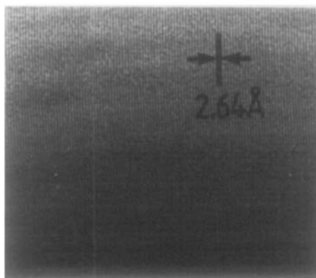
FIG. 5. Extended perfect crystal of \text{SnO}_2 from sample B with strong one-dimensional lattice fringes of 2.64-Å spacing.
