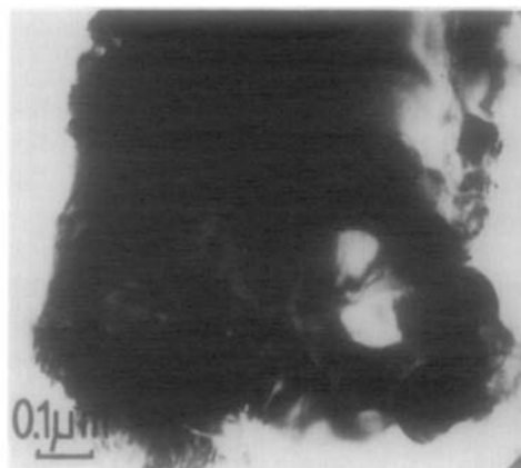
FIG. 13. Region of tin-antimony oxide G showing a number of small crystals apparently embedded in a large crystal.
