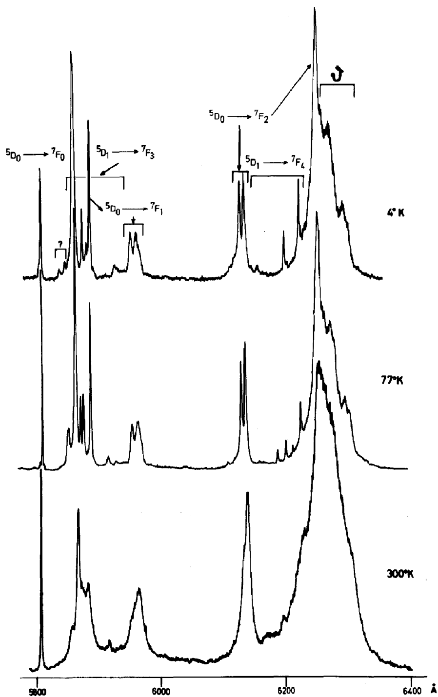
FIG. 1. Emission spectra of Eu 3+ : La 2 O 3 (1%) at 4, 77, and 300 K under uv excitation ( \nu = vibronics).
