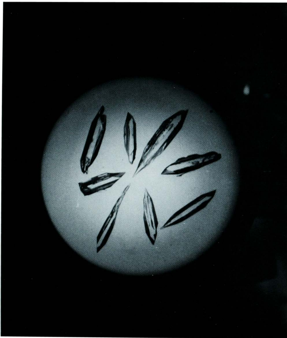
FIG. 1c. Crystal morphology of \text{NH}_4\text{CeP}_4\text{O}_{12} (monoclinic).
