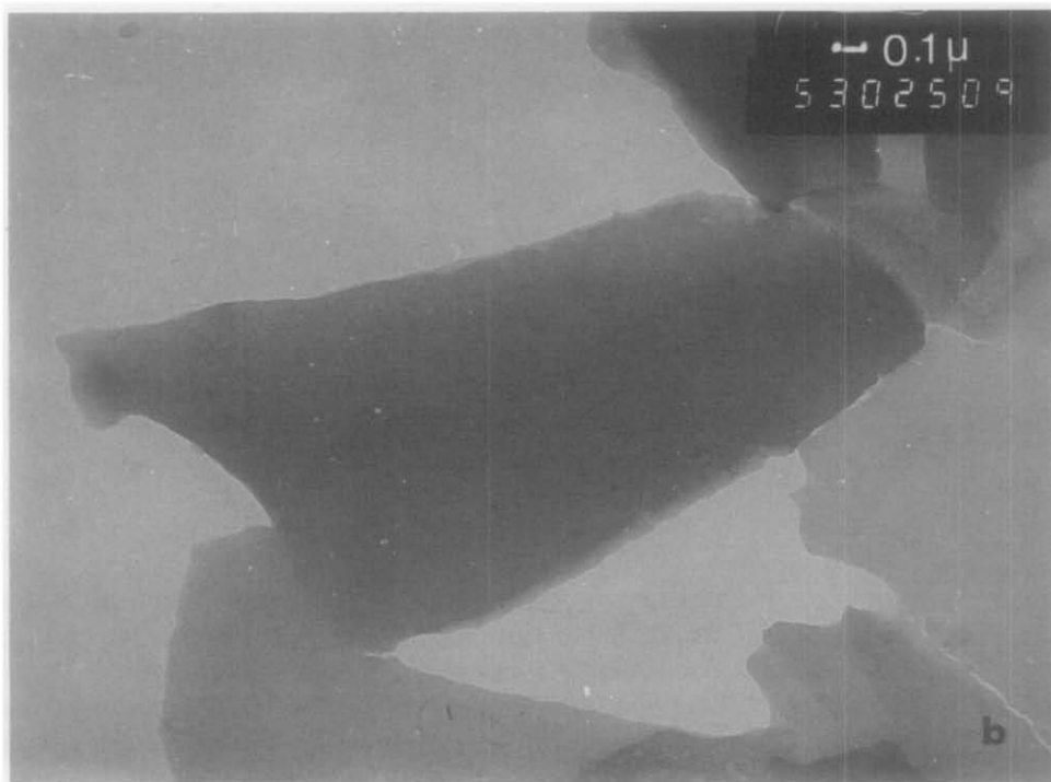
FIG. 4. TEM micrographs of particles of colloidal \text{VOPO}_4 \cdot \text{H}_2\text{O} : (a) general view; (b) crystallite corresponding to diffraction (c); (c) diffraction diagram; (d) UHR diagram.
