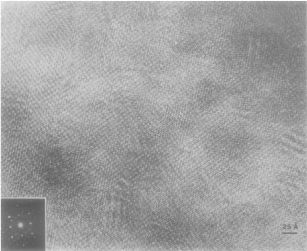
FIG. 10. A high-resolution image of a region of the alloy film in Fig. 9. The formation of \text{SnO}_2 is indicated by the Debye rings in the diffraction pattern. The image of the alloy having a composition of \text{AuSn}_2 consists of 6 \times 6 -Å fringes with extensive finer contrast with some moiré fringes probably caused by overlapping \text{SnO}_2 particles.
