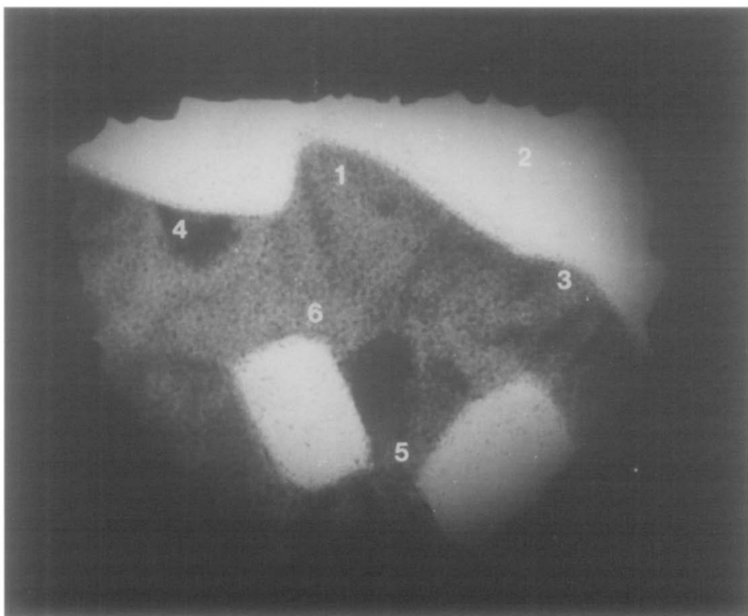
FIG. 9. An image of a thin alloy film with the numbered microanalysis sampling regions. Mottling of the film surfaces and the contamination layer is the result of the electron-beam-induced formation of \text{SnO}_2 particles.
