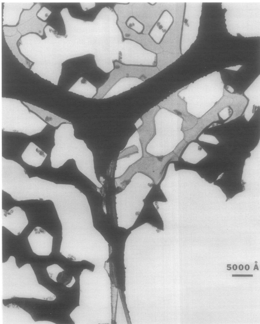
FIG. 3. A two-film arrangement of gold and tin films showing the effects of heating at 200°C for 10 min. The grayish areas represent amorphous layers left behind by the recession of the tin films.
