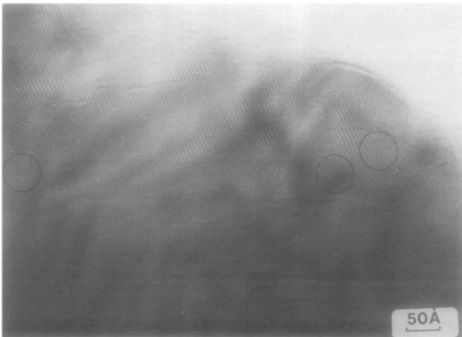
FIG. 8. High-resolution image of a region showing disorder of the structure; lattice fringe system is unidimensional in this part of the crystal. (001) plane.
