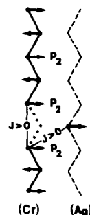
FIG. 7. Ferromagnetic coupling ( J ) between uncompensated spins for \text{Ag}_{1/2}\text{Cr}_{1/2}\text{In}_{(1/2-x)}\text{PS}_3 ( x \leq 0.20 ).
