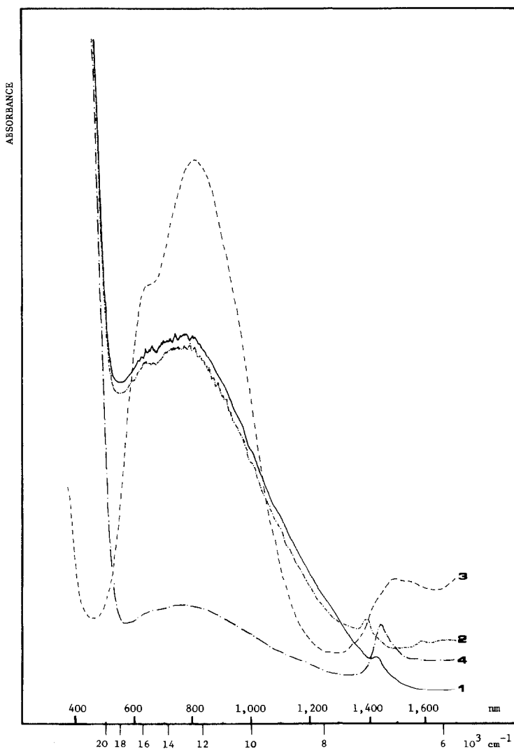
FIG. 4. UV-visible spectra of (1) P_1 , (2) P_2 , (3) \text{VOHPO}_4 \cdot 0.5\text{H}_2\text{O} ( \text{V}^{4+} content), (4) \text{VOPO}_4 \cdot 2\text{H}_2\text{O} ( \text{V}^{5+} content, with a few having a quantity of \text{V}^{4+} due to \text{H}_2\text{O} interaction).
