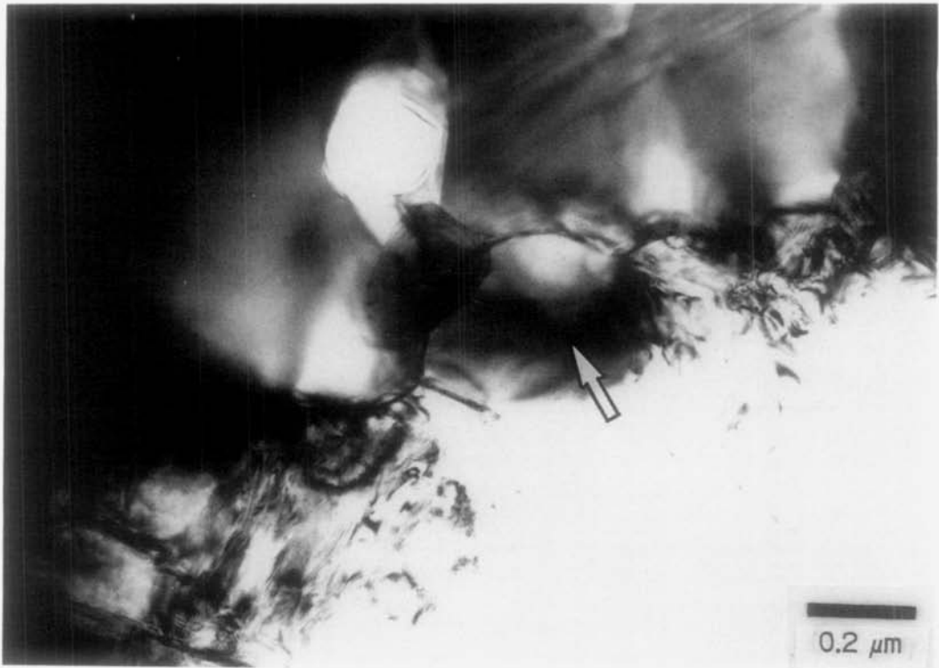
FIG. 2. Micrograph of 30 mole% \text{ZrO}_2 -70 mole% \text{ZrN} compound, with the X phase indicated by an arrow.
