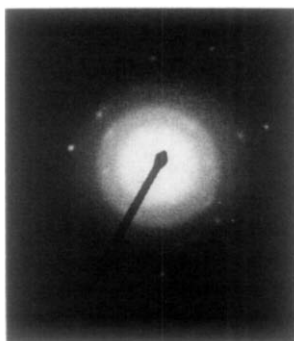
FIG. 5. ED patterns of specimens showing a complete destruction of the structure with the appearance of an amorphous state.
