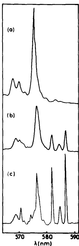
FIG. 4. Influence of the Ca/Ln ratio on the optical absorption spectrum of \text{Nd}^{3+} \ ^4I_{9/2} \rightarrow \ ^4G_{5/2}, \ ^4G_{3/2} hypersensitive transition at 4 K. The beam is parallel to the c axis of the crystals. Starting compositions: (a) \text{Ca}_{0.7}\text{Nd}_{0.3}\text{Mg}_{0.3}\text{Al}_{11.7}\text{O}_{19} (CLnA), (b) \text{Ca}_{0.3}\text{La}_{0.67}\text{Nd}_{0.03}\text{Mg}_{0.7}\text{Al}_{11.3}\text{O}_{19} (CLnA), (c) \text{La}_{0.9}\text{Nd}_{0.1}\text{MgAl}_{11}\text{O}_{19} (LNA after (6)).
