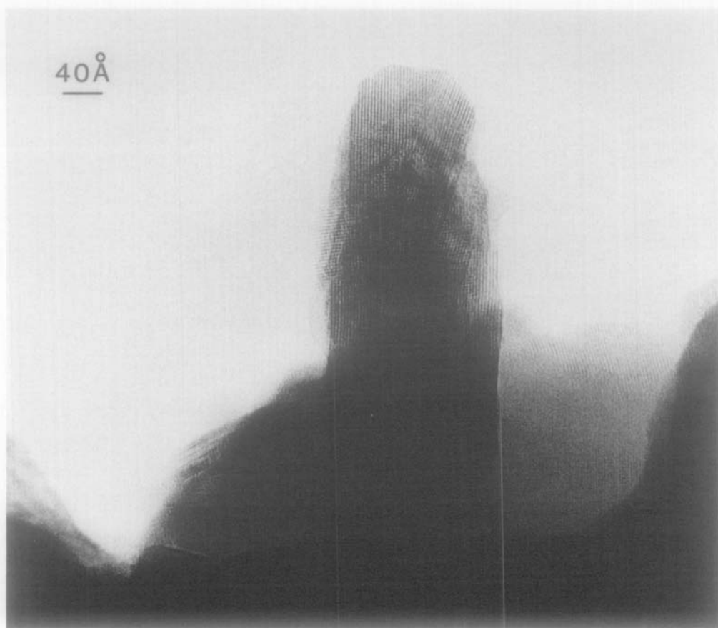
FIG. 6. An image illustrating the growth habit of the precipitating crystal. The principal growth direction is (011) but the crystal is clearly faulted.
