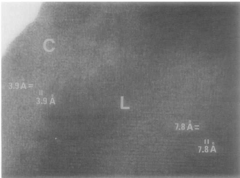
FIG. 3. Corresponding electron micrograph showing L twin domains intergrowth with a cubic perovskite (C).
