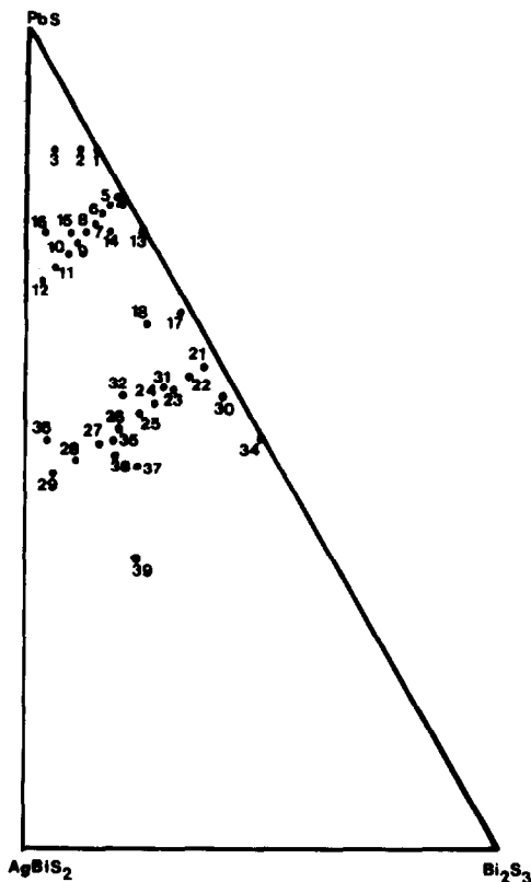
FIG. 2. Diagrammatic representation of the compositions studied. The numbers correspond to the preparations detailed in Table II.
