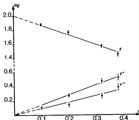
FIG. 4. Evolution with composition of the number of normal F, relaxed  $F''$ , and interstitial  $F'''$  anions for the  $\text{Ca}_{1-x}\text{La}_x\text{F}_{2+x}$  solid solution ( $0.10 \leq x \leq 0.38$ ).
