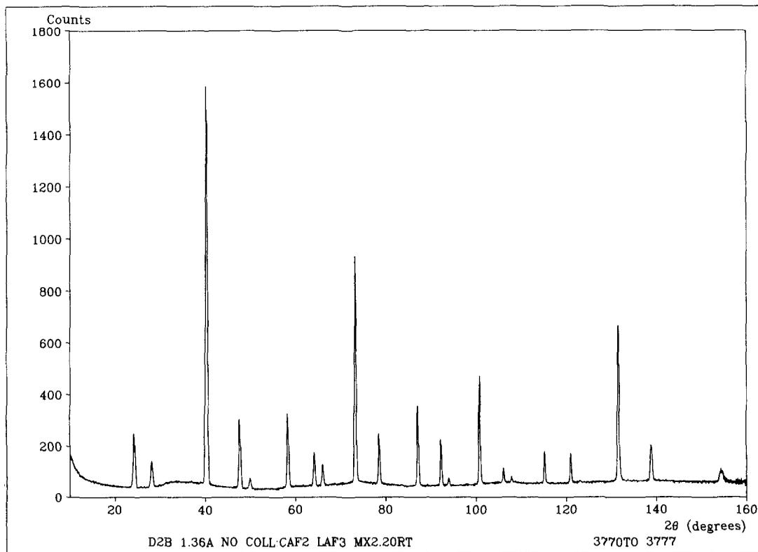
FIG. 2. Diffraction pattern at room temperature of the  $\text{Ca}_{0.80}\text{La}_{0.20}\text{F}_{2.20}$  sample (D2B diffractometer).
