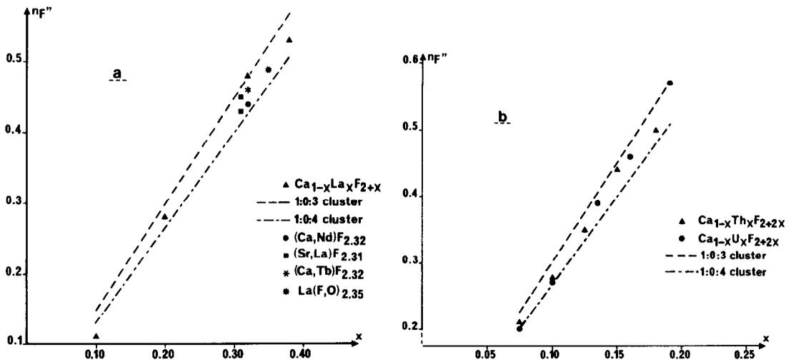
FIG. 5. Comparison of experimental  $n_{F''}$  with theoretical ones (1:0:3 and 1:0:4 clusters) for (a)  $M_{1-x}Ln_xF_{2+x}$  phases ( $M^{II} = \text{Ca, Sr}$ ). The two values given for the  $(\text{Sr, La})F_{2.31}$  compound correspond to different refinement conditions (see Ref. (20)). (b)  $\text{Ca}_{1-x}M_x^{IV}F_{2+2x}$  phases ( $M^{IV} = \text{Th, U}$ ).
