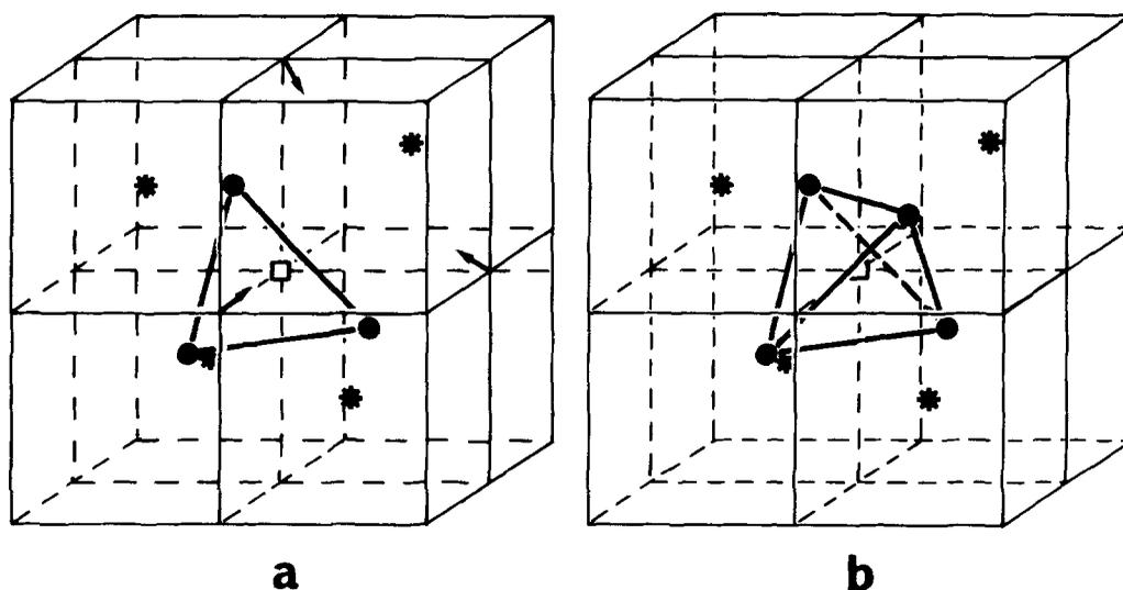
FIG. 1. Schematic views of two 1:0: $n$  clusters: (a) the 1:0:3 cluster; (b) the 1:0:4 cluster (cubic basis vectors are parallel to edges of the cubes and origin is at a cation site). \*, Cations; ●,  $F''$  interstitials; □, anion vacancy. Small arrows show the  $F \rightarrow F''$  relaxation in the 1:0:3 cluster.
